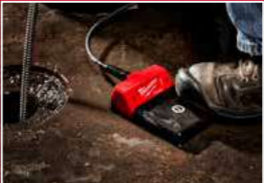
Electronic foot pedal with non-slip grip
