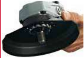
Tool-free quick release safety guard
