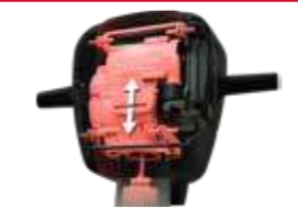
Milwaukee® floating body AVS system enables to lean the tool against the body without feeling the vibrations
