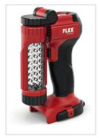
Powerful LED worklamp with 24 cold-white LEDs and integrated discharge protection. LED head can be swivelled through 320° and folded through 180°. Swivelling and lowerable hook for attaching the lamp and belt clip. Lighting duration: approx 20 hours with 2.5 Ah battery pack and approx 40 hours with 5.0 Ah battery pack. FLEX battery system: suitable for all 18 V battery packs. Delivery does not include battery.
