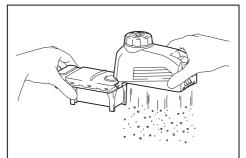
3. Dispose of the dust, and then clean the filter.
