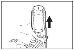
**NOTE:** If the cap comes off from the dust cup, attach it with its printed side facing up so that groove on the cap fits in the inside periphery of the attachment.
