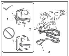
1. Double looped portion of the hook 2. Lanyard (tether strap) 3. Locking carabiner (multi-action and screw gate type)
