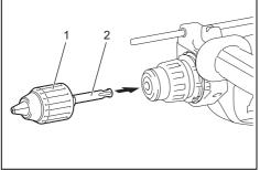
1. Keyless drill chuck 2. Chuck adapter
