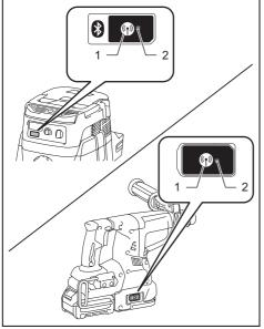
Wireless activation button 2. Wireless activation lamp If the cancellation is performed successfully, the wireless activation lamps will light up in red for 2 seconds and start blinking in blue.
